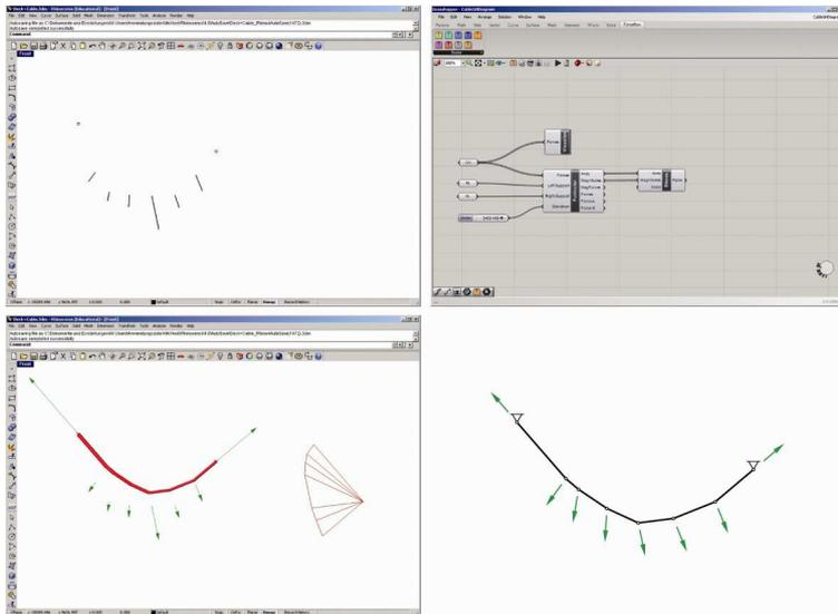
Fig. 2: The funicular component. Input: lines as forces and points as supports, and rise as real number (left above). Parametric definition: Funicular component and two components for visualization of inner and external force (right above). Output: funicular polygon, force diagram, reaction forces (left below). Structural system: kinematic (right below).
