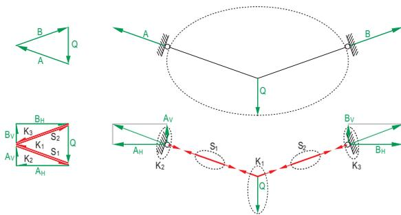
Fig. 1: Form and force diagram of a hanging cable for one node (above); joined diagrams for three nodes (below); from [6], p. 17
