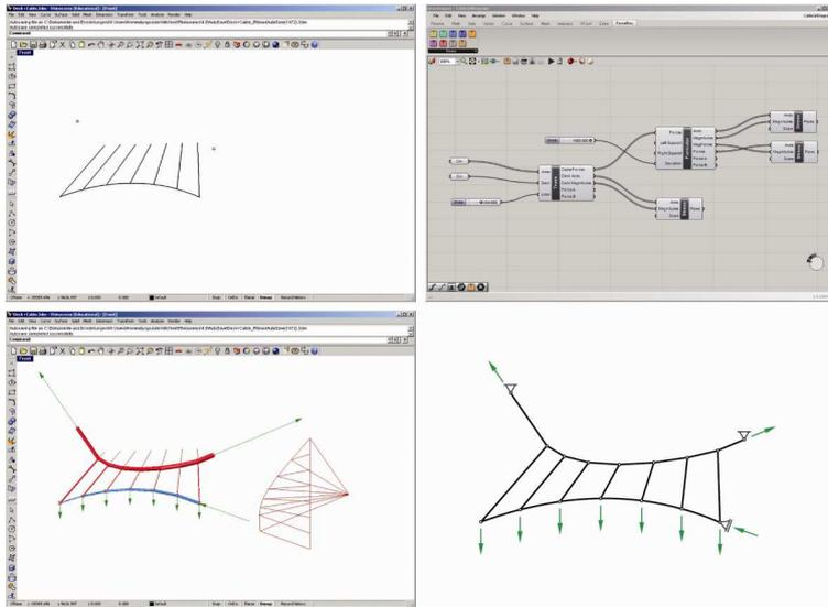
Fig. 4: The system combined from the cantilever and the funicular system: Input: deck curve, hanger axes, supports of the funicular as points (left above). Parametric definition: merged definition of the cantilever and the funicular (right above). Output: reaction forces and joined force diagrams (left below). Structural system: kinematic (right below).
