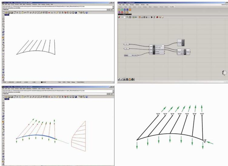
Fig. 3: The cantilever component. Input: curve as deck, variable number of lines as force axes, numerical load magnitude (left above). Parametric definition: cantilever component, and two components for visualization of inner and external force (right above). Output: force diagram, reaction forces (left below). Structural system: determinate (right below).
