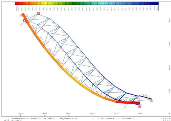
Fig. 7: Result of the FEM analysis, based truss elements that can only transfer axial forces
