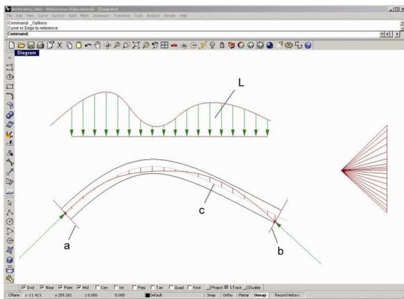
Fig. 5: Elastic line of thrust for a given arch and loading
